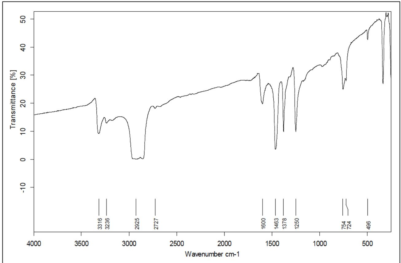
Figure 1. IR spectrum of Diamminedichloropalladium
