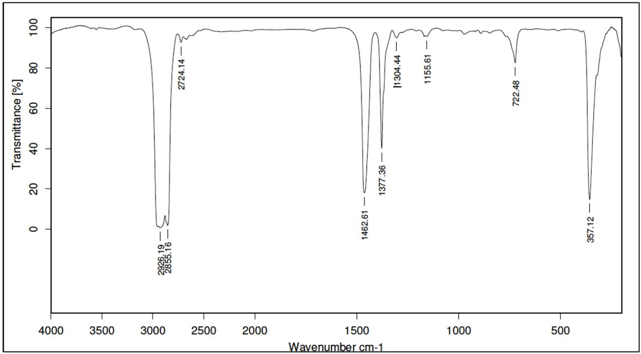
Figure 1. Typical infrared spectrum of dipotassium hexachloropalladate
